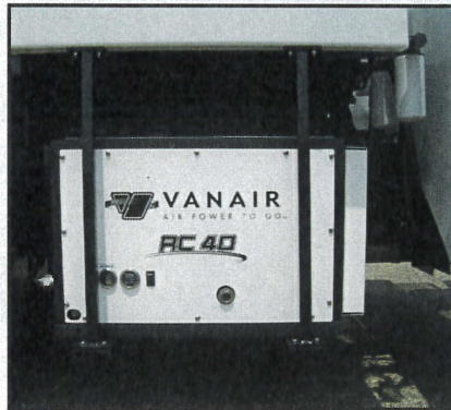
Hydraulic Vanair Compressor
