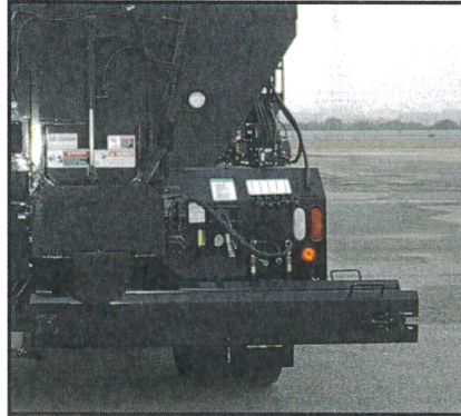
Side Dumping Conveyor
